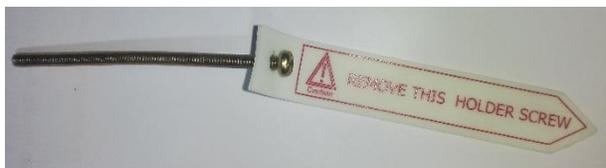
Before connecting the camera, Open it and remove the holder screw, which is located on the side of the lens.
